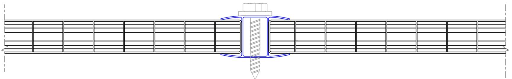
DETALLE DE ENCAJE CON PERFIL "H" 16 mm
