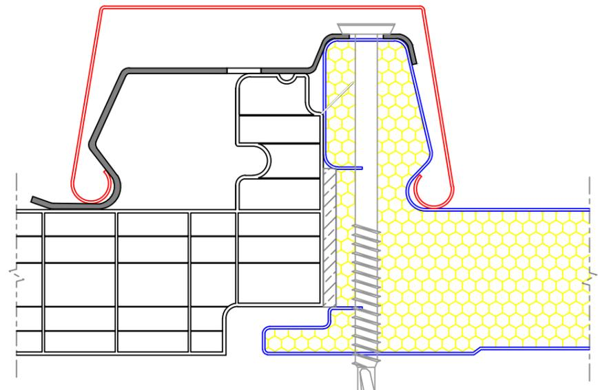
DETALLE DE ENCAJE CON PANEL DE POLIURETANO DE 30mm
