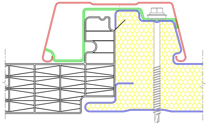
DETALLE DE ENCAJE CON PANEL DE POLIURETANO DE 30mm
